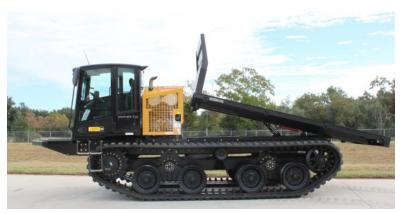
Built with a truck-inspired widened chassis to accept virtually all implements without any modifications, the PANTHER T12 is pictured here with a tilting flat bed. From construction to right-of-way maintenance, in the middle of nowhere or within city limits, both the PANTHER T8 and the T12 have the toughness, tenacity and reliability you need in a crawler.
